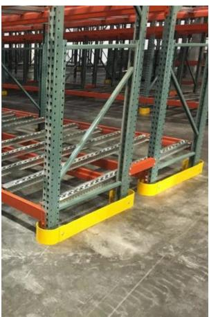
K3 End-of-Row Guards are built to protect standard 42" and 48" deep pallet racks.
